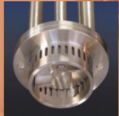
The **Slotted Head** provides the most popular combination of high shear and efficient flow rates. It is well-suited for emulsions and many medium-viscosity mixing applications.
