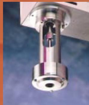
**Model 100 ILC: 1 HP** – An in-line rotor/stator generator converts the 100LC Laboratory High Shear Mixer to an in-line mixer with excellent versatility in the lab. The in-line unit is available with either a standard single-stage rotor/stator or a four-stage QuadSlot design for higher shear rates. With a mechanical seal, it can operate under vacuum or pressure.
