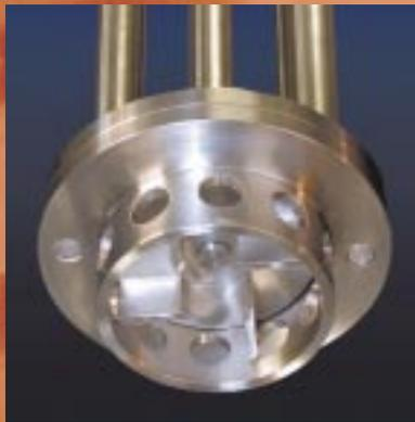
The **Disintegrating Head** is excellent for general purpose mixing, fast particle size reduction of larger solids, and vigorous flow.
