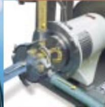
The In-line SLIM system replaces older design concepts that relied on an additional pump and eductor. In the In-line SLIM unit, solids are combined with the liquid stream and instantly subjected to intense shear – with no need to pump the solids downstream from the eductor to the mixer. The result is far greater capacity and less clogging.
