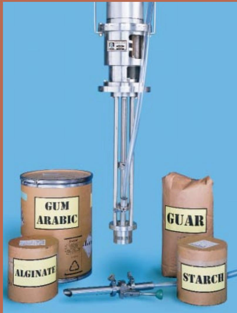
**Model 505 Stainless Steel High Shear Mixer with batch SLIM system: 5HP** – While the mixer is running, the operator simply inserts the feed tube into a container of powder and opens the feed valve. The vacuum created by the specially modified rotor/stator generator draws the powder through the tube and directly into the high shear zone. Dusting and delays are eliminated.
